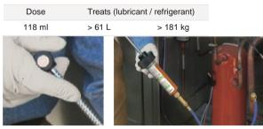
Inject dye with a turn of the handle.
